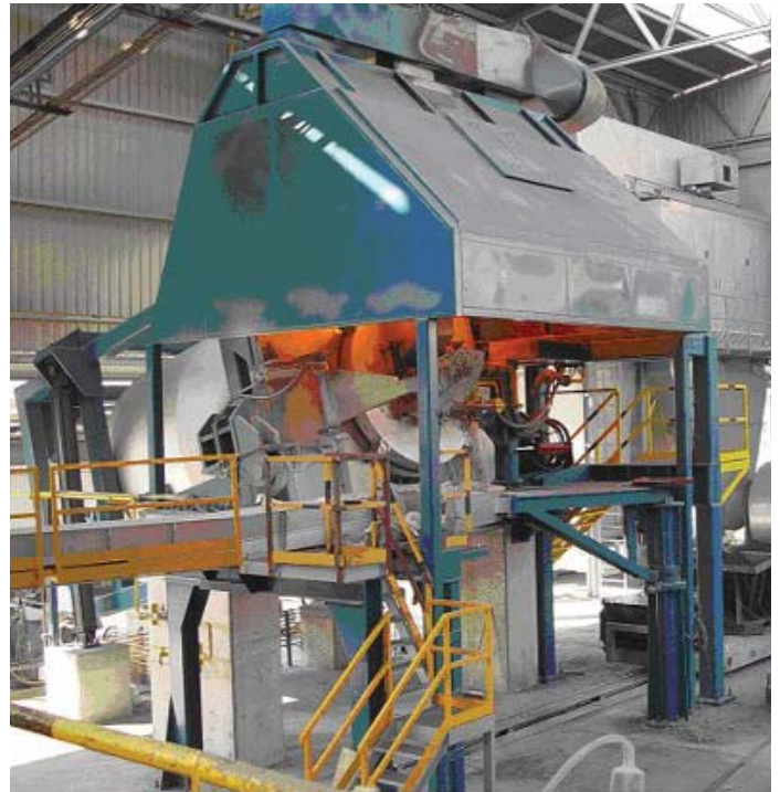
ALTEK-MDY 16 tonne tilting type rotary furnace
