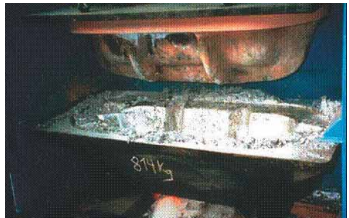
4 Dross Press in operation
