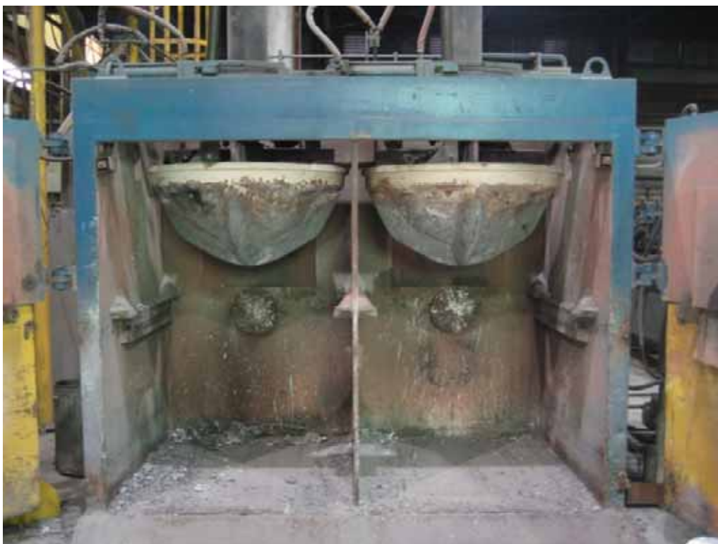
Internal view of the press showing the patented ribbed 701 head
